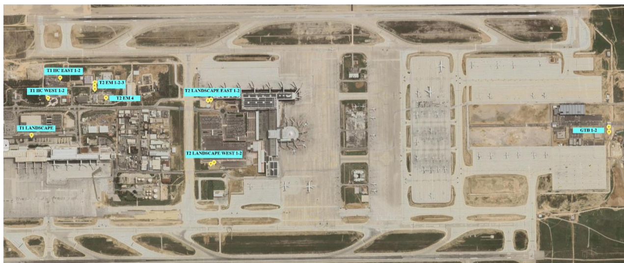
Figure 2. Groundwater wells at Fraport TAV Antalya Airport
